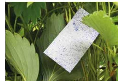
Picture 3: Strategically placed water sensitive paper provides an analysis of the spray coverage effectiveness Left = Good Right = Poor
